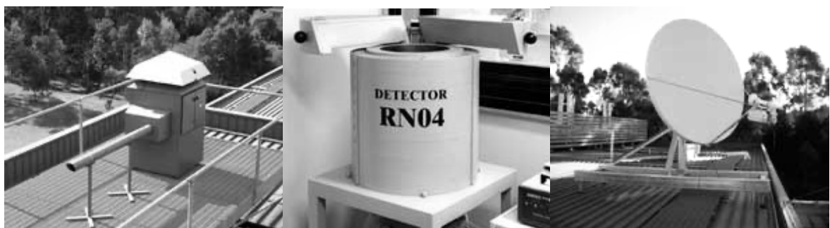
Figure 30—Components of a radionuclide monitoring station: (left) particulates are sampled from the air onto a filter; (centre) the filter is analysed with a high sensitivity detector; and (right) data on radionuclides measured are forwarded to Vienna where they are compiled and released to CTBT signatories. Photos courtesy of ARPANSA.
